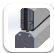
End Cap Between Wall and Panel
